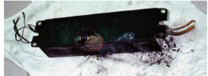
Burnt PCB Light Ballast
